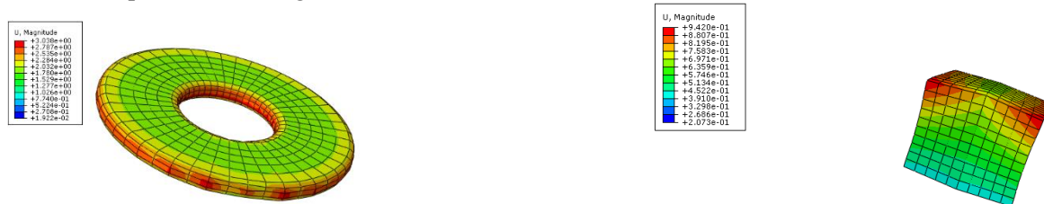
Figure 3. Shows FE model of compression tests and results. (a) FE model of silicone rubber gasket and (b) deformation of an embedded sensor.
