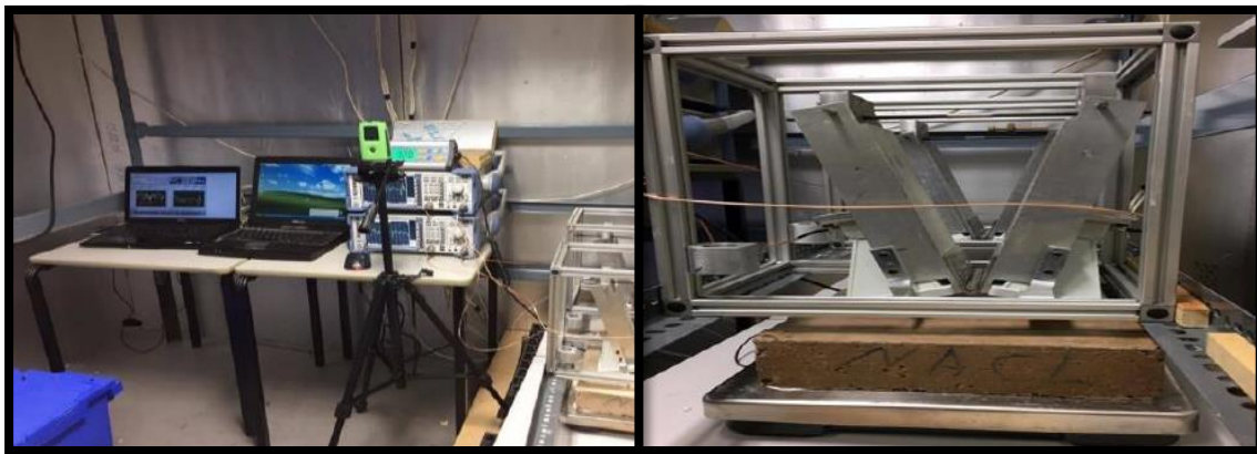
Fig. 2: S_{21} Measurements of drying off process slab for 72 hours (salt water)
