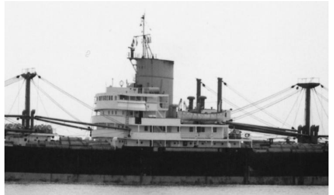
m.v. 'PATANI' mid to Late 1960's (EDL Livery) New Funnel, Signal/Radar Mast. - Topmast, Triatic Stay and 'log' boom removed. After mast & king Post no longer painted black to disguise funnel soot.
