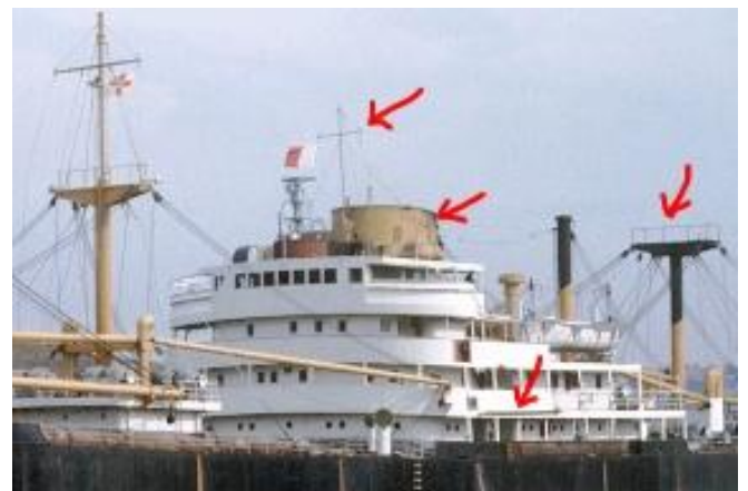
m.v. PATANI (light ship) UK after June 1963 with scaffolding signal mast conceived and built by Cadet Steve New & the Ch. Officer in March 1963
