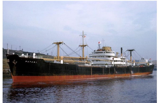
m.v. PATANI (light ship) UK after June 1963 with scaffolding signal mast conceived and built by Cadet Steve New & the Ch. Officer in March 1963
