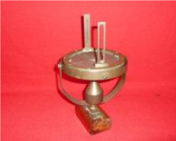
Pelorus for taking relative bearings. m.v. 'PATANI' had no bridge wing gyro repeaters.
