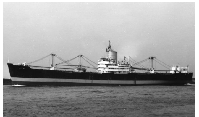
m.v. 'PATANI' Late 1960's (Ocean/EDL Livery) New Funnel, Signal/ Radar Mast, Topmast Removed
